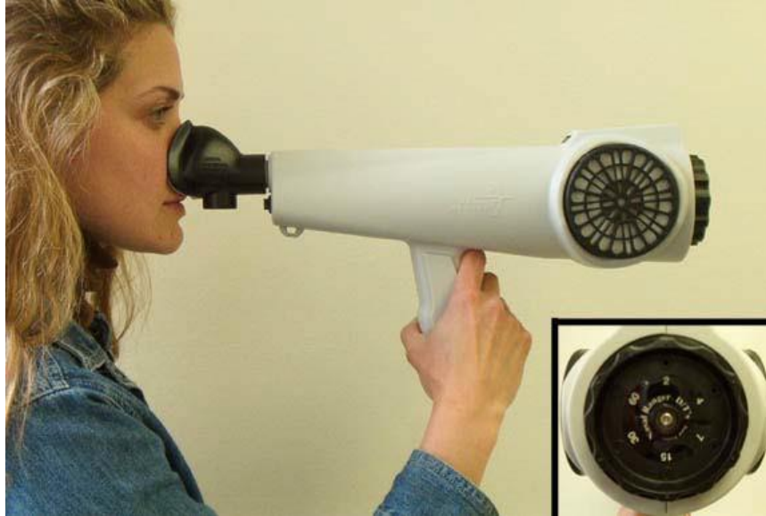
Figure 4.3. The Nasal Ranger® Field Olfactometer (St. Croix Sensory, Inc.). The inset picture shows a close-up of the orifice dial, which is located at the right side of the Nasal Ranger in this photo.
