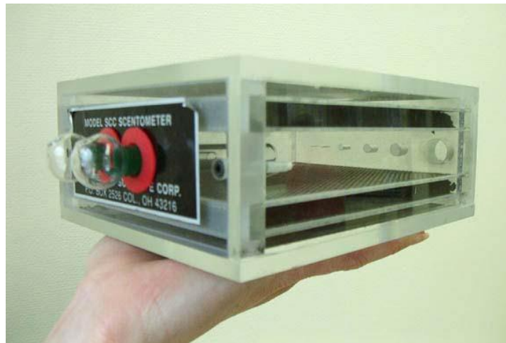
Figure 4.2. The Scentometer Field Olfactometer (Barnebey Sutcliffe Corp.). Note the two glass nostril ports to the left and the series of orifice holes at the back of the unit to the right in this photo.
