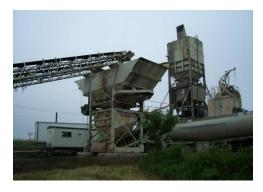
Unless there are multiple conveyors or front-end loaders feeding the bins or multiple front-end loaders feeding the conveyors, it can be assumed that only one type of material is being loaded into the bins at a time. The DNR recommends the weighted average emission rate from filling the bins with aggregate and sand be used. Alternatively, a conservative estimate can be determined by using the emission rate for filling the bins with aggregate only.
