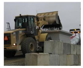
hopper and the bottom of the bucket of the front-end loader as it dumps the material into the hopper. The initial horizontal dimension ( $\sigma_y$ ) is the square-root of the lateral area of the hopper divided by 4.3. The initial vertical dimension ( $\sigma_z$ ) is the distance the material falls from the bucket of the front-end loader to the top of the hopper divided by 2.15.
