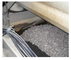
This source is eliminated at some facilities by weighing the material in the elevated storage bins directly and then drawing off until the weight of the material remaining in the bins equals the original weight minus the weight of the material required for the batch. In these cases, the DNR recommends the emissions from the unloading of the elevated storage bins onto the conveyor that feeds the truck loadout or central mixer be added to the sources that represent the elevated storage bins.
