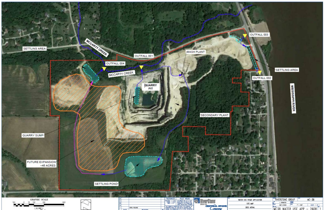
Figure 1: Map of applicant's site including the quarry pit, sump pit, wash plant, settling ponds, outfalls, water pathways, and future expansion area.
