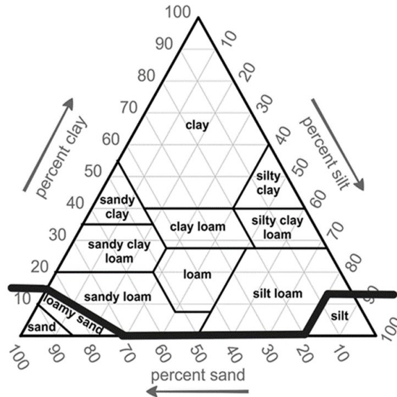
USDA textural classification chart. Sand size particles, 2-0.05 mm; silt-sized particles, 0.05-.002 mm; and clay sized particles, less than .002 mm.
