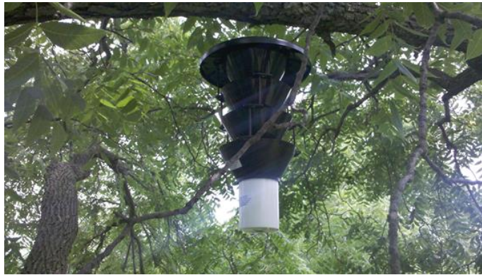
Figure 11. One of the Lindgren funnel traps that were used in conjunction with the walnut twig beetle pheromone. The traps were placed at sawmills, communities, and campgrounds. (Image: Shane Donegan, DNR)
