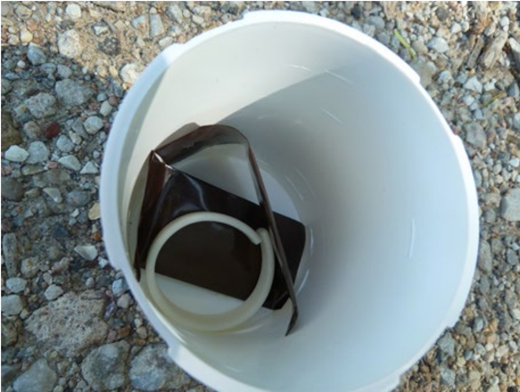
Figure 12. A look inside the Lindgren Funnel trap capture chamber. The picture shows two pheromone pouches and a 3 inch long strip of dog collar that was used to kill the beetles that entered the capture chamber. (Image: Shane Donegan, DNR)
