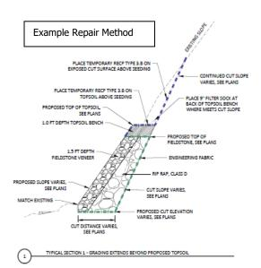
In the fall of 2024, DNR hired Bolton and Menk to further assess these bank collapses and complete engineering design to stabilize the toe of the slope at critical sites. This project aimed to address stabilizing the base of the slope at the water's edge to prevent future erosion.
