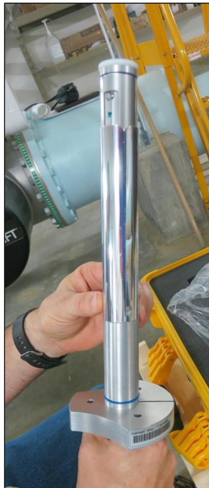
UV Light used for *Cryptosporidium* Inactivation
