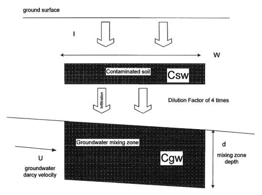
Csw: concentration in the soil water Cgw: concentration in the groundwater
