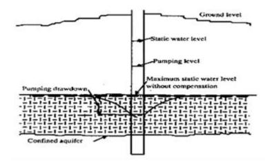
(4) Protected levels for flowing wells will be considered the top of the confined aquifer or 100 feet below the surface, whichever is higher. Flowing wells shall be constructed to accommodate a pump capable of supplying a sufficient water supply at protected levels.
