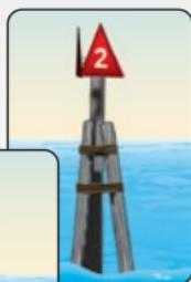
**Daymarks** are permanently placed signs attached to structures, such as posts, in the water. Common daymarks are red triangles (equivalent to nuns) and green squares (equivalent to cans). They may be lighted also.
