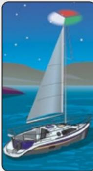
An alternative to the sidelights and sternlight is a combination red, green, and white light, which must be exhibited near the top of the mast. The red over green and white combination lighting may also be used. (Not shown in picture.)
