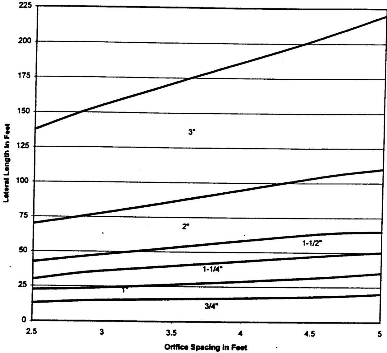
Fig. A -3b. Minimum lateral diameter based on orifice spacing for 1/4 in. diameter orifices (Wisc. Dept. Of Commerce, 1999).
