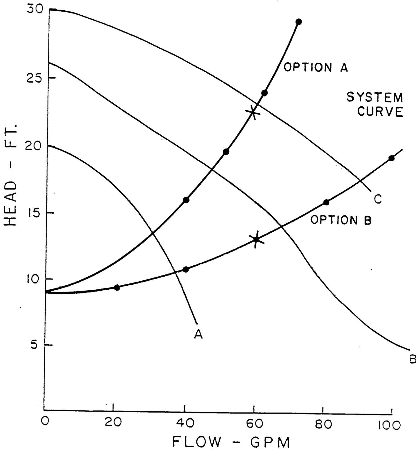
Fig. A-4 System performance curve and several pump performance curves for the example problem. For this example, the pump must provide a flow of at least 60 gpm
