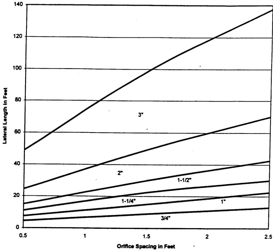
Fig. A -2b. Minimum lateral diameter based on orifice spacing for 3/16 in. diameter orifices (Wisc. Dept. Of Commerce, 1999).
