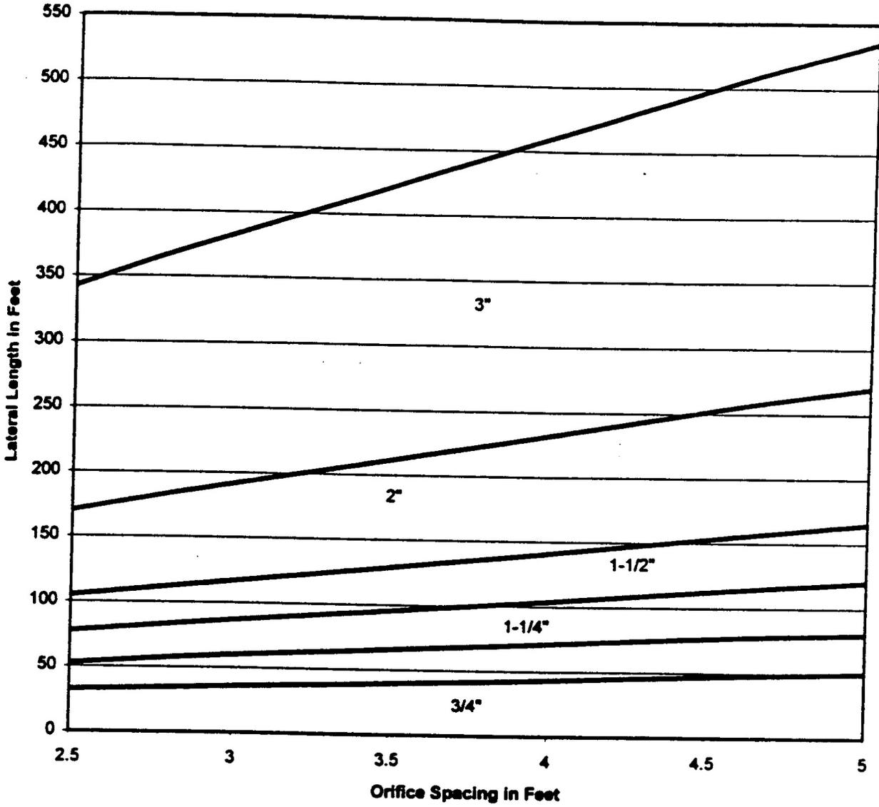
Fig. A -1b. Minimum lateral diameter based on orifice spacing for 1/8 in. diameter orifices (Wisc. Dept. Of Commerce, 1999).
