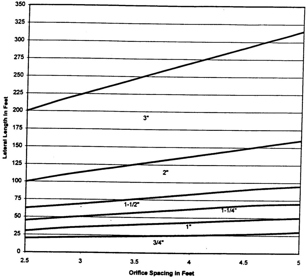
Fig. A -2a. Minimum lateral diameter based on orifice spacing for 3/16 in. diameter orifices (Wisc. Dept. Of Commerce, 1999)
