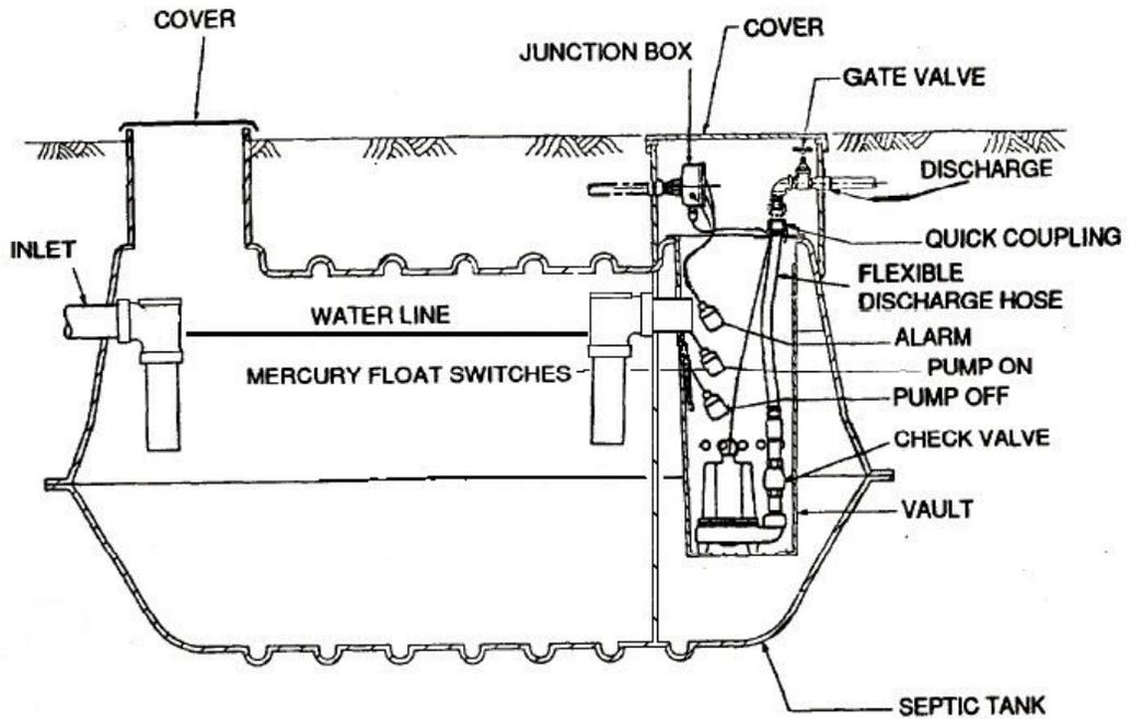
Figure 3-3 Centrifugal STEP pump and internal pump vault (EPA, 1991)
