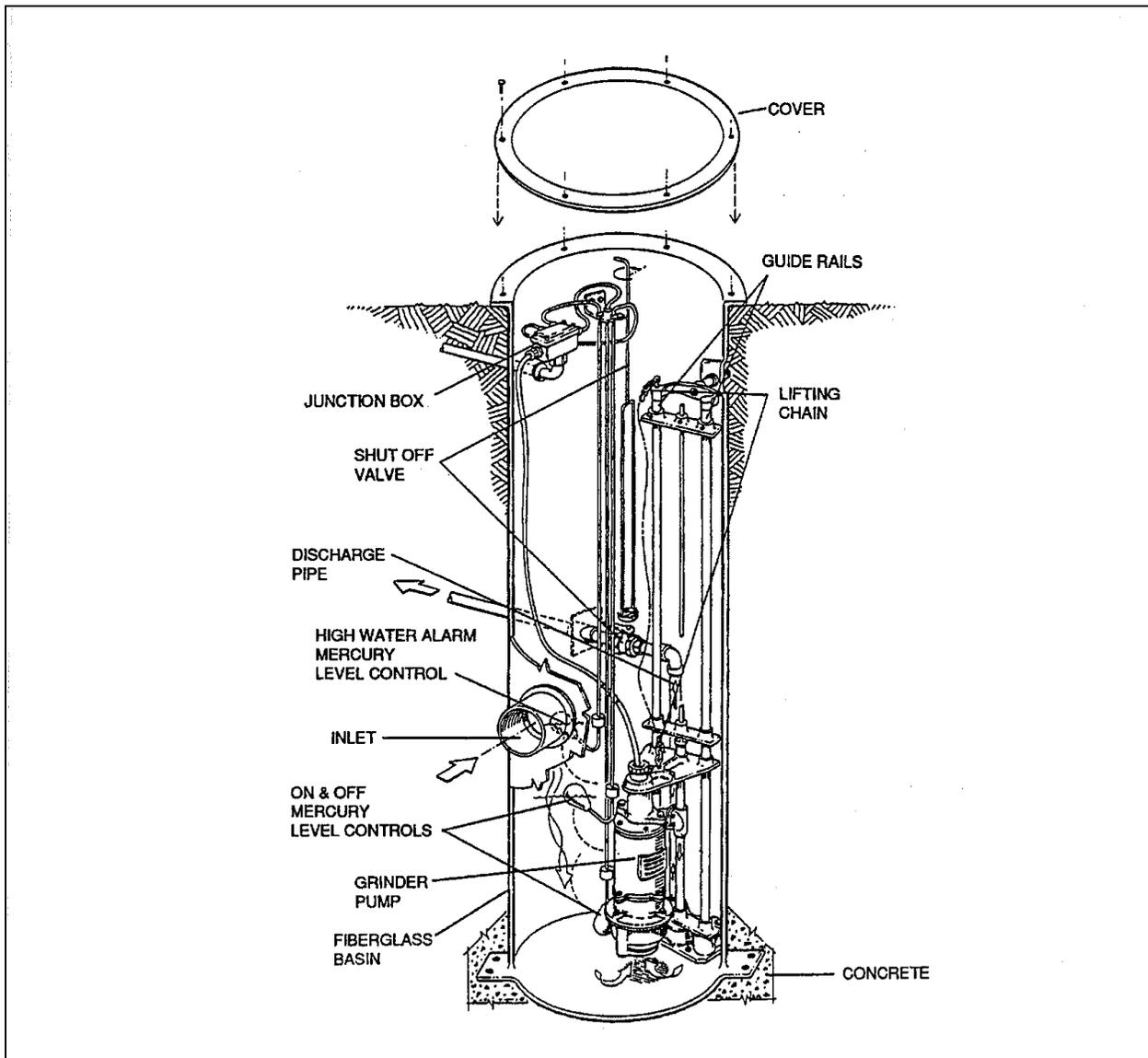
Figure 5-2 Typical Centrifugal Grinder Pump installation (Courtesy F.E. Myers/Pentair Water).
