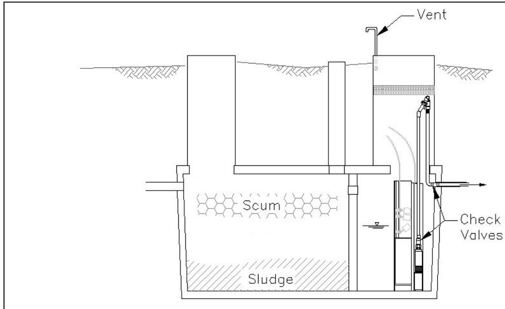
Figure 3-2 Two-compartment septic tank with turbine-style (Orencia, Inc.) pump.
