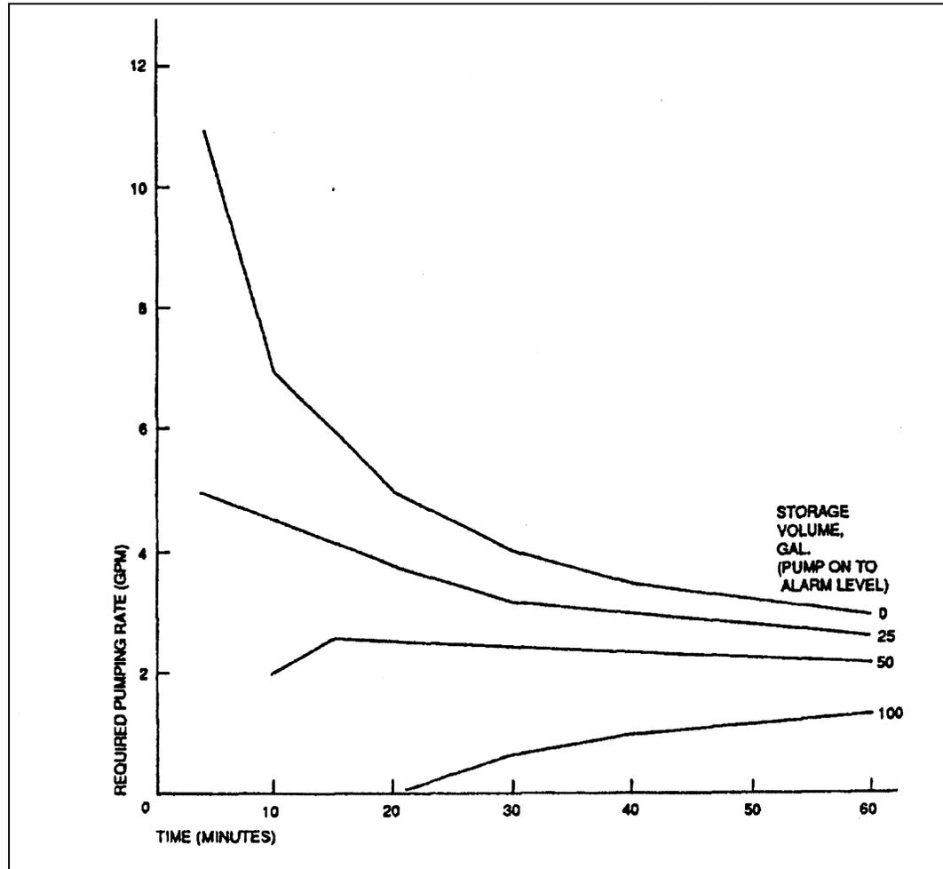
Figure 3-8 Required pumping rates based Reference 11, <1% regression
