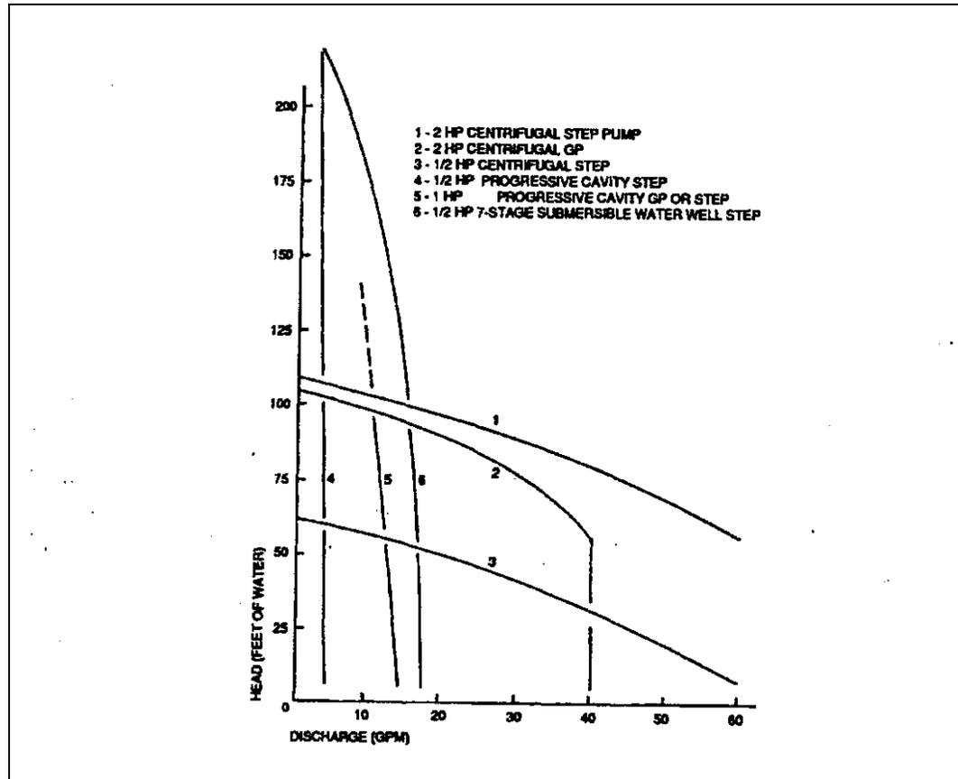
Figure 3-6 Discharge curves for pumps used in pressure sewers (EPA, 1991)
