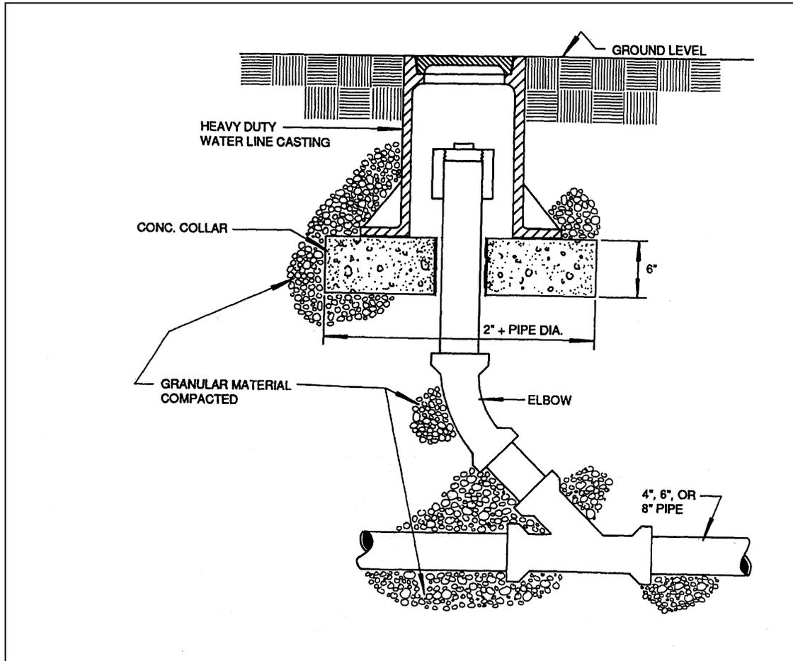
Figure 4-1 Typical STEG cleanout detail (EPA, 1991)
