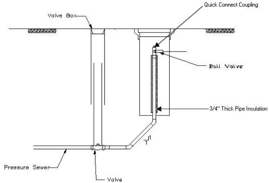
Figure 3-9 Typical single-flush connection
