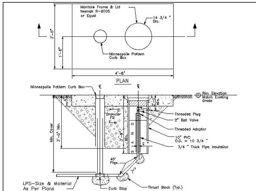
Figure 3-10 Typical single-flush connection.
