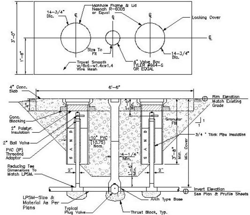
Figure 3-11 Typical dual -flush connection.
