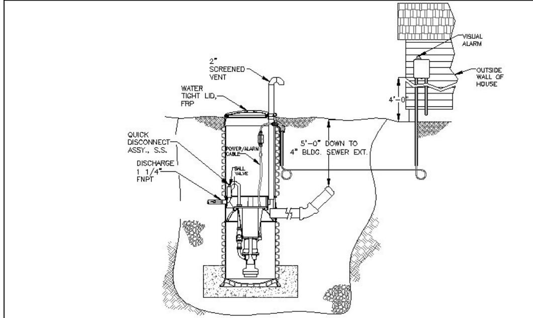
Figure 5-4 Typical Progressing Cavity Grinder Pump installation
