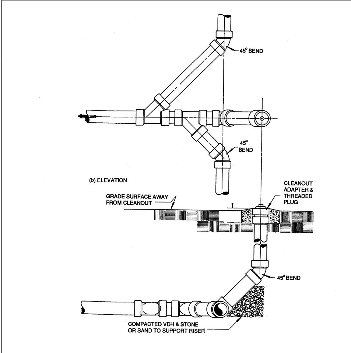
Figure 4-2 Typical STEG cleanout detail (EPA, 1991)
