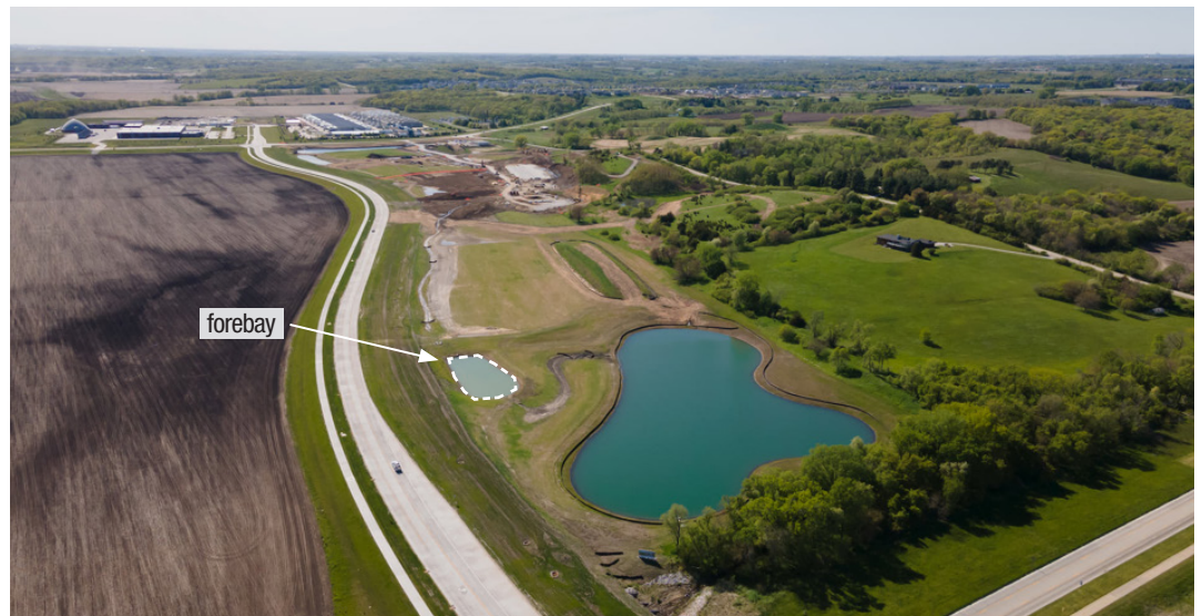
Wet forebay during site construction. West Des Moines, IA.
