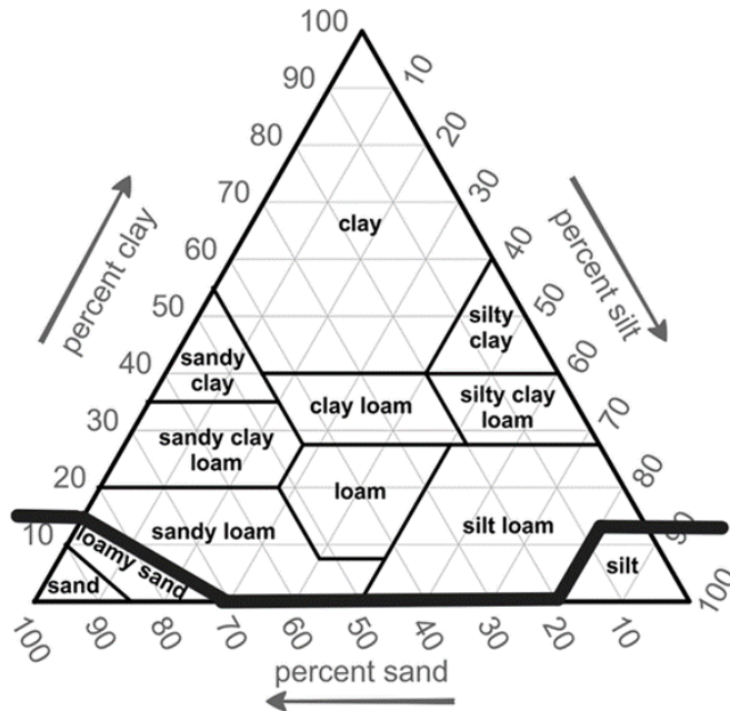
U.S.D.A. textural classification chart. Sand size particles, 2-0.05 mm; silt-sized particles, 0.05-.002 mm; and clay sized particles, less than .002 mm.
