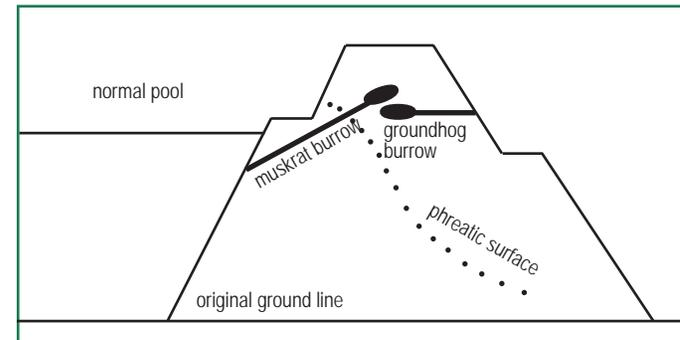
Figure 2: Dangerously close rodent burrows cause a hazard to earth dams.
