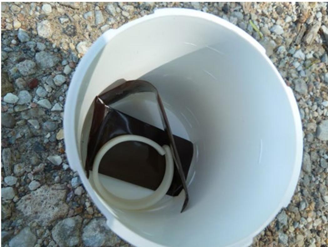
**Figure 13. A look inside the Lindgren Funnel trap capture chamber. The picture shows two pheromone pouches and a 3 inch long strip of dog collar that was used to kill the beetles that entered the capture chamber. (Image: Shane Donegan, DNR)**
