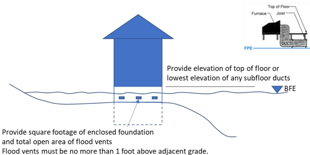
**Type D: Floodproofed Construction (only allowed for non-residential structures).**
