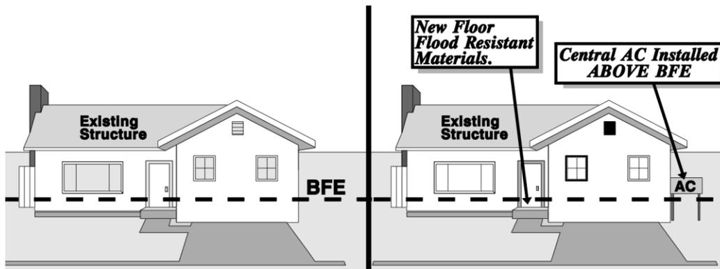
**Figure 12-3 Minor rehabilitation using flood-resistant methods and materials**
