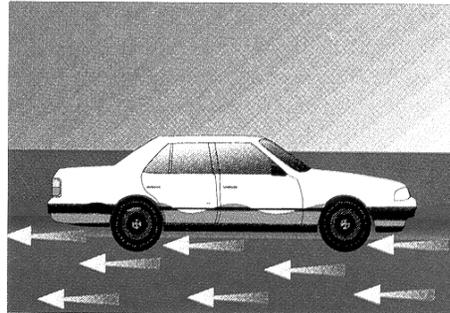
When a vehicle stalls in the water, the water's momentum is transferred to the car. For each foot the water rises, 500 lbs. of lateral force are applied to the car.
