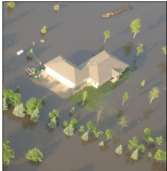
**Figure 11-2 A new building elevated on fill plus freeboard was not damaged by this flood**
