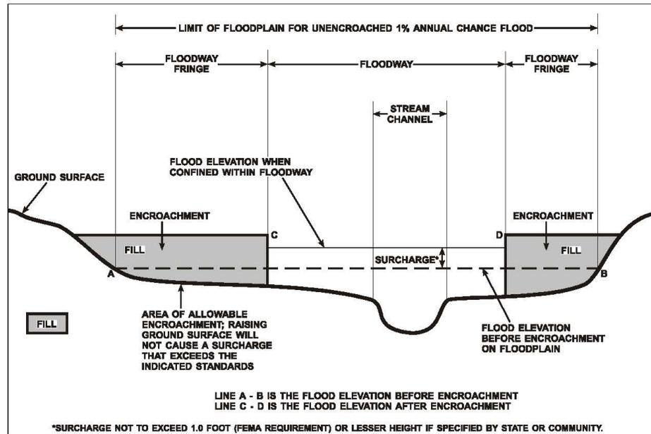
Figure 1 - Floodway Schematic
