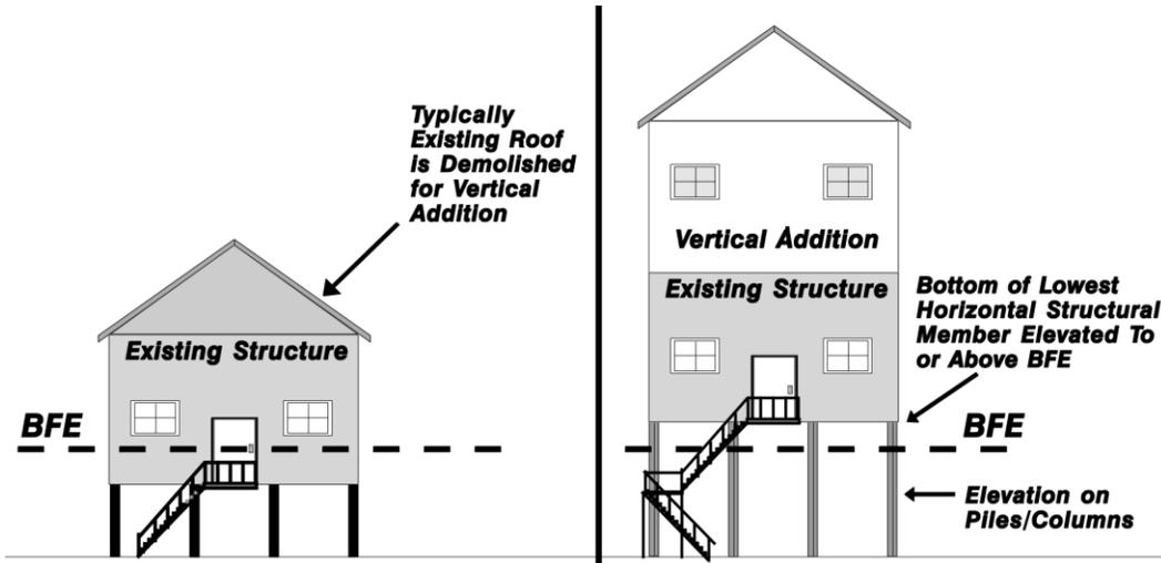
Figure 12-7 Vertical addition to a residential building
