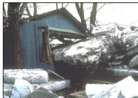
**Figure 13-11 Ice floes and other large items of debris can crush a house**
