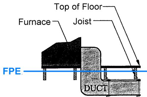
**Figure 11-6A** Just focusing on getting the lowest floor above the flood protection elevation (FPE) means that floor joists and ductwork may still be flooded.
