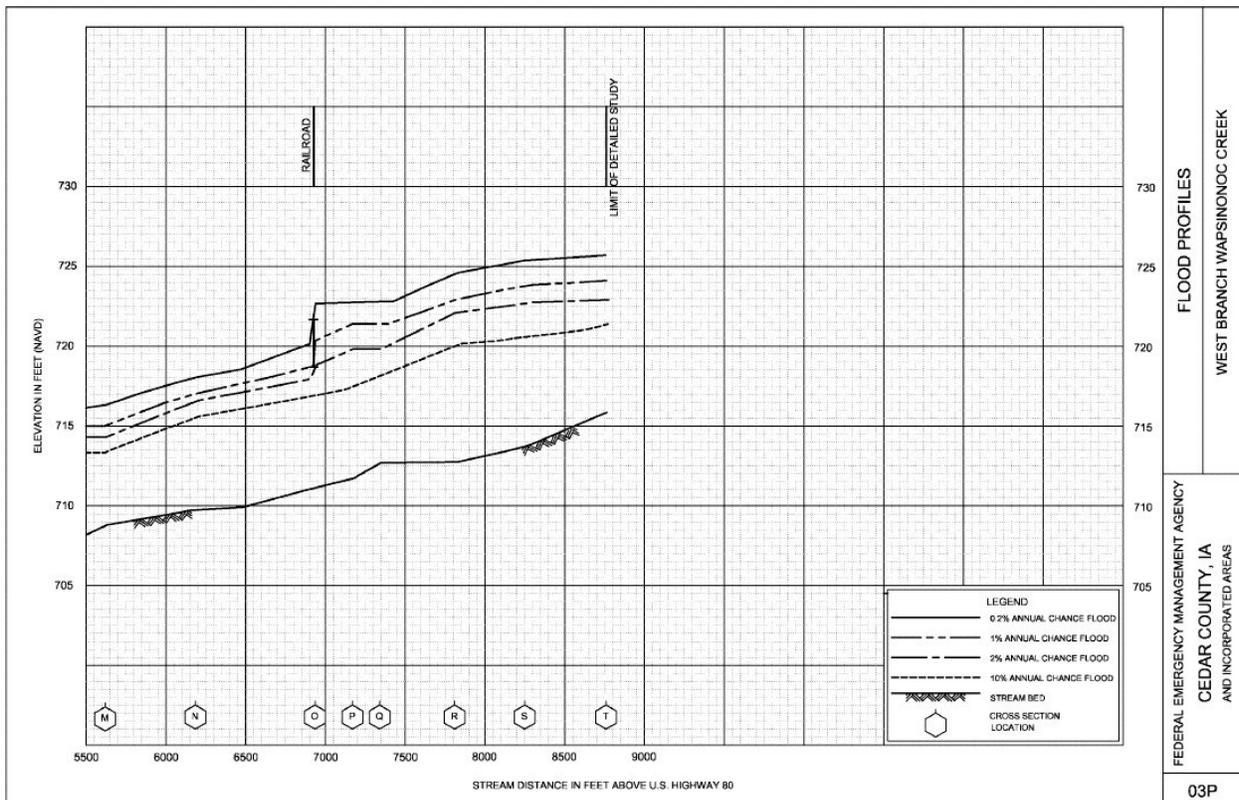
Figure 3-6 Flood profile for West Branch Wapsinonoc Creek
