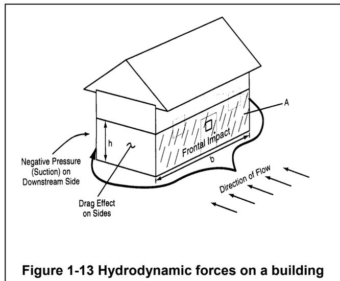
The speed of moving water is called **velocity**, a movement that is usually measured in feet per second. The faster water moves, the more pressure it puts on a structure and the more it will erode stream banks and scour the earth around a building's foundation.
