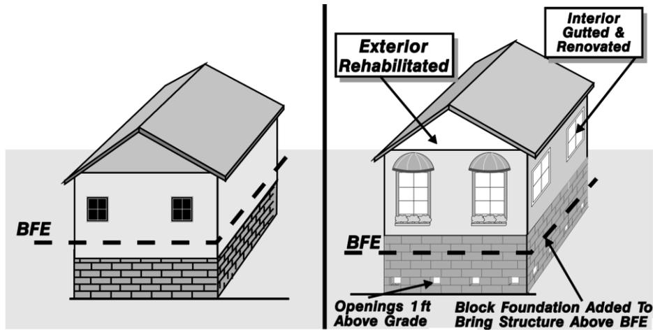
Figure 12-4 Substantially rehabilitated building elevated above the BFE
