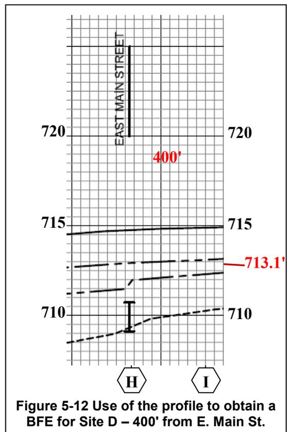
Figure 5-12 Use of the profile to obtain a BFE for Site D – 400' from E. Main St.
