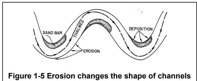
Figure 1-5 Erosion changes the shape of channels
