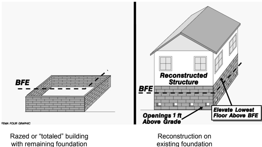
Figure 12-14 A reconstructed house is new construction
