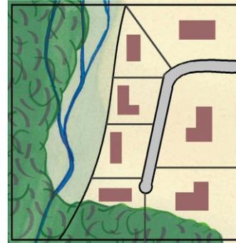
Figure 7-3 Example of well-designed subdivision plan building site out of SFHA
