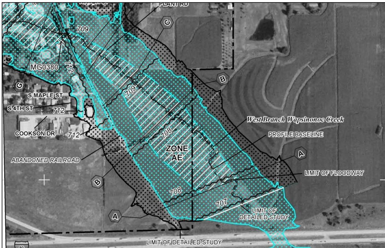
**Figure 10-3 Example floodway on a countywide Flood Insurance Rate Map (FIRM)**
