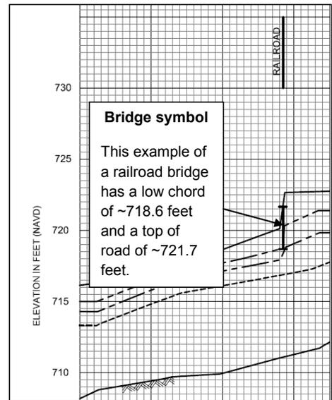
Figure 3-5 Profile showing bridge symbol
