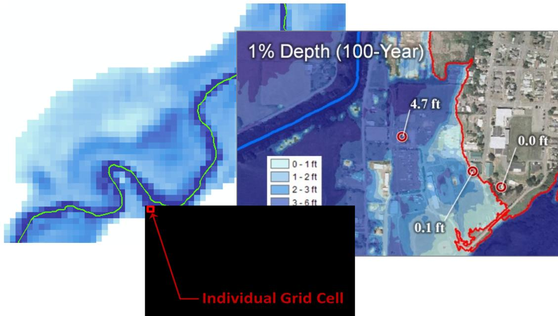
Figure 3 Example of a mapped depth grid
