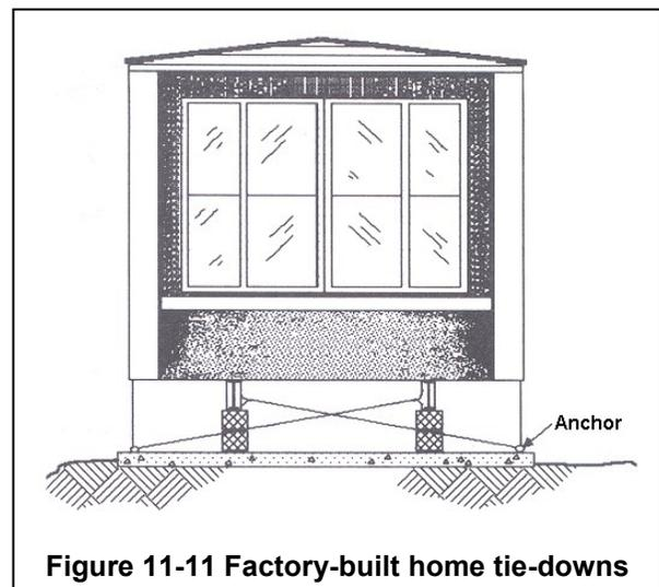
“Adequately anchored” means a system of ties, anchors, and anchoring equipment that will withstand flood and wind forces. The system must work in saturated soil conditions. Usually this means over-the-top or frame tie-downs in addition to standard connections to the foundation.
