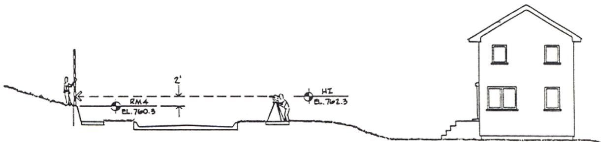
Figure 15-6 Starting elevation (760.3) + reading on rod (2') = height of instrument (HI) = 762.3
