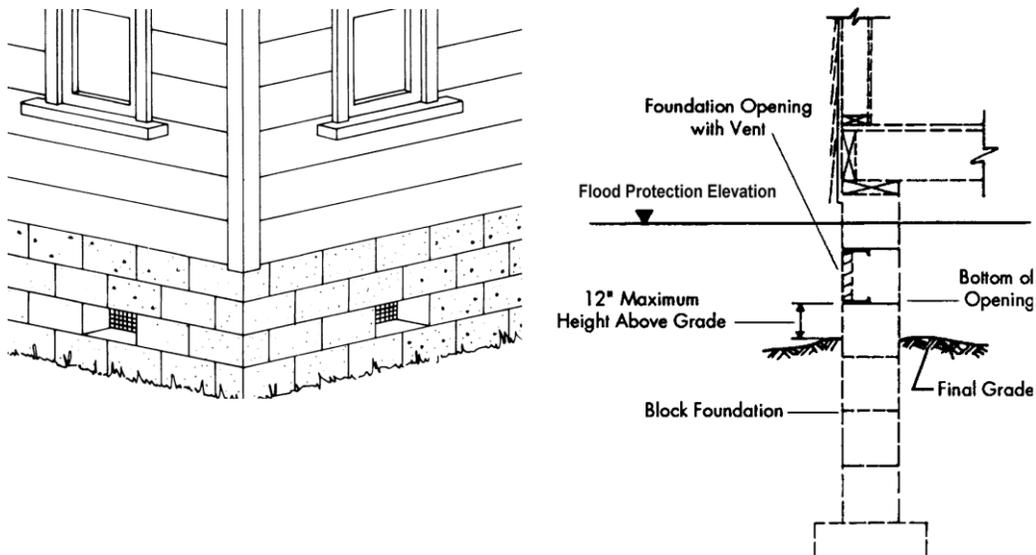
**Figure 11-7 Opening location in solid foundation wall**
