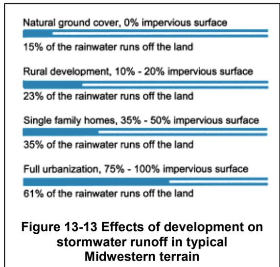
One way to reduce the impact of stormwater from new development is to require the developer to restrict the rate at which the increased runoff leaves the property. The developer must build a facility to store stormwater runoff on the site. Unfortunately, stormwater detention only manages the rate of release of the water—it does nothing about increased volumes of water due to decreases in permeable surfaces.
