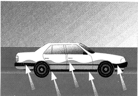
But the biggest factor is buoyancy. For each foot the water rises up the side of the car, the car displaces 1,500 lbs. of water. In effect, the car weighs 1,500 lbs. less for each foot the water rises.
