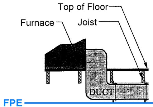
**Figure 11-6B** A properly elevated building has all damageable items, including floor joists, furnace, and ductwork, above the flood protection elevation (FPE). The ductwork could also be run overhead, through the attic.
