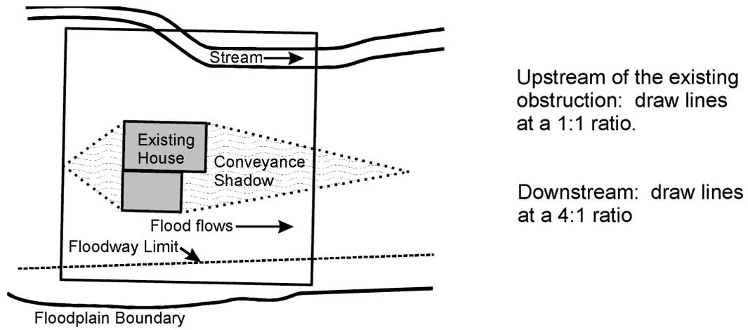
**Figure 10-7 Determining the conveyance shadow**
