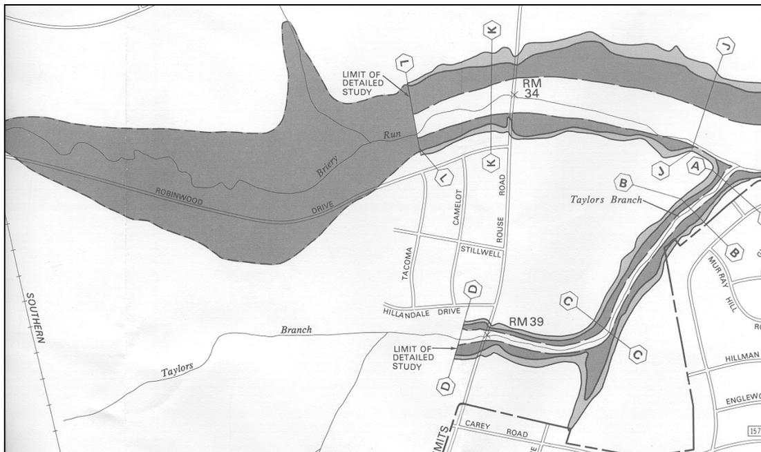
Figure 4-12 FBFM showing floodway, cross sections, and SFHAs
