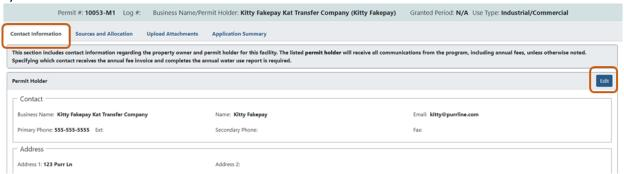
6. Navigate to the Sources and Allocation tab of the application. If applicable, make any requested changes to the sources listed on the permit, or the individual wells/intakes listed under each source. Use the Edit Source button to change the amount or rate requested for an individual source.
