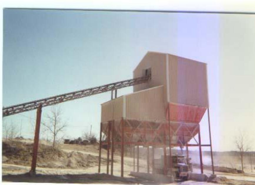
**Figure 1. Example loadout operation. (Trinity Consultants, 2004)**
