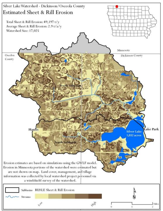
Figure 12. Relative sheet and rill erosion rates in the Silver Lake watershed.
