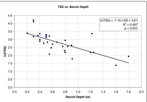
Figure 5. Regression of In(TSS) versus Secchi depth.
