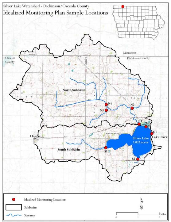
Figure 14. Idealized monitoring plan sample locations.
