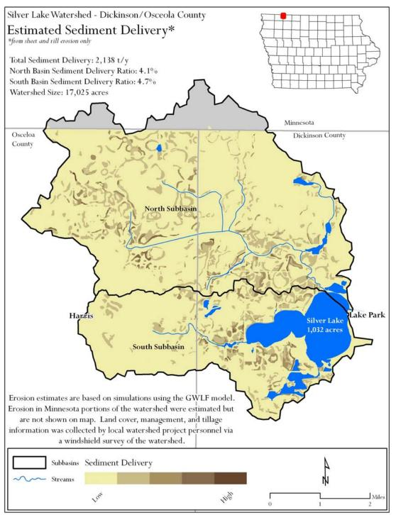
Figure 13. Relative sediment delivery ratio (SDR) in the Silver Lake watershed.
