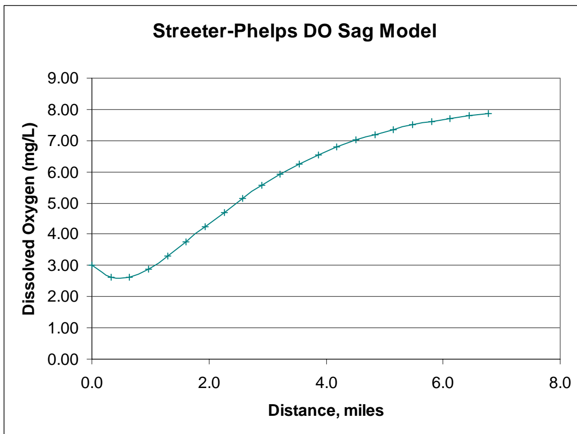
Figure 2. Sanborn WWTP Streeter Phelps Model Oxygen Sag Curve.
