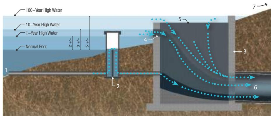
1. 1st Stage: Small Diameter Inlet - Low Flow Control (Below Surface)
