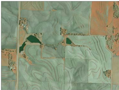
2002: Terraces and retention ponds reduce erosion and sediment reaching the stream.
