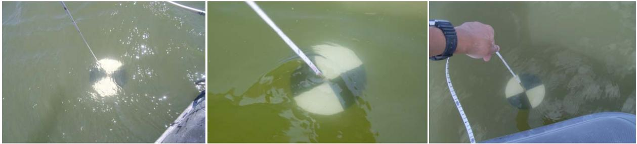
Figure 7. Secchi transparency photos (disc at 0.2 m depth) at site RA-3 from left to right: early summer, mid-summer, and late summer. Average Secchi depth in 2013 was 0.5 m. Photos courtesy of ISULL.
