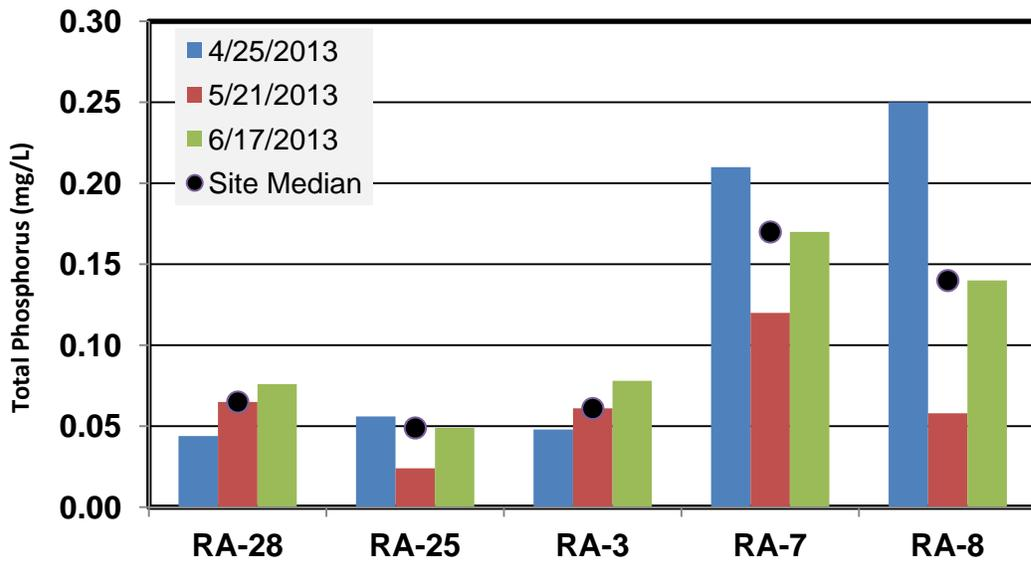
Figure 8. Total phosphorus concentrations at USACE monitoring sites for April – June 2013. Courtesy of USACE.
