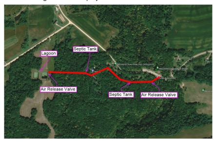
needing constant maintenance due to excessive amount of debris getting into the sewer system. There are two old air release valves that are currently malfunctioning and the sewer lines are in need of jetting and cleaning.
