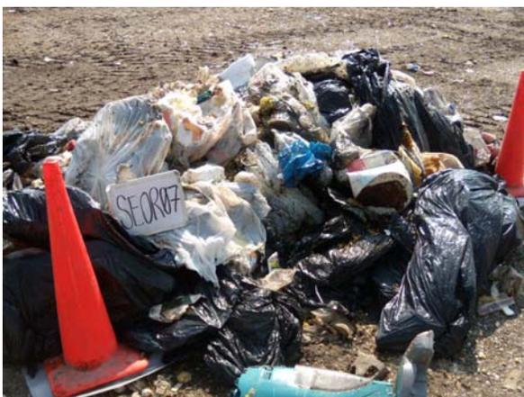
Once the area of the tipped load was selected, the Field Supervisor coordinated with a facility-provided loader operator to take a “grab” sample of wastes from that point in the tipped load. The loader operator removed a sample of waste that exceeded the targeted sample weight, and placed the grab sample in a secure area to await sorting. Each was labeled by its identifying number using a white board. This is shown in Figure 2-2. The white board for sample identification stayed with
