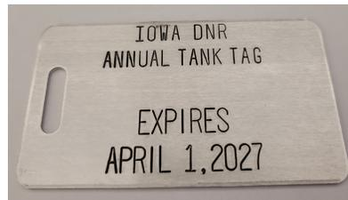
An annual tag listing "April 1, 2027" is required to receive fuel for tanks greater than 1100 gallons. The annual tag listing "April 1, 2027" must be on the UST fill port to receive fuel deliveries.
