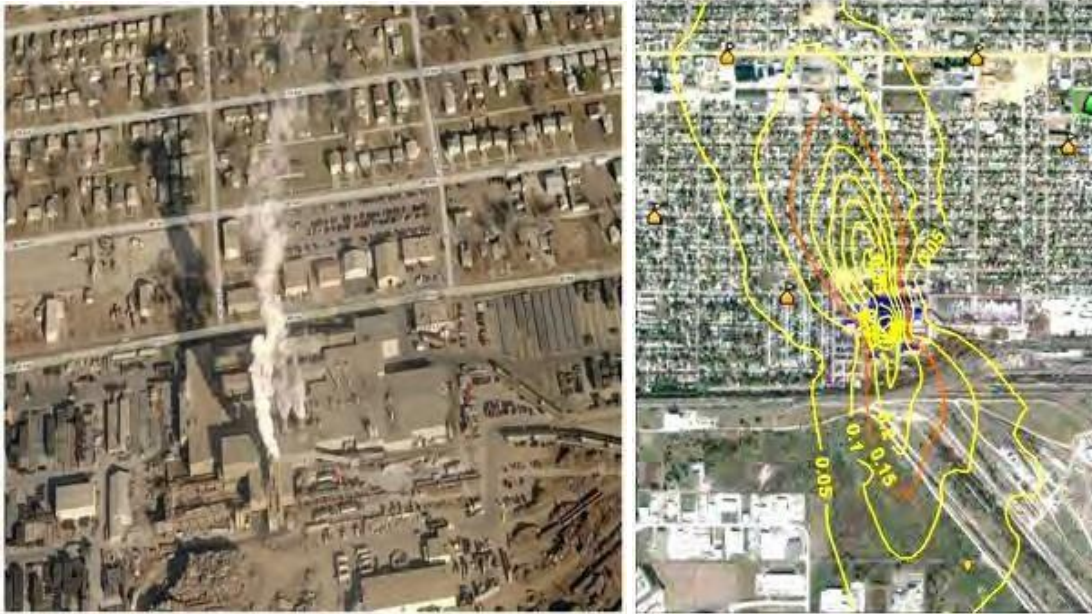
Local Air Pollutant Example. Industrial Lead Emissions (Left), and Modeled Hotspot (Right). The Area inside the Orange Contour is Predicted to Violate the NAAQS.
