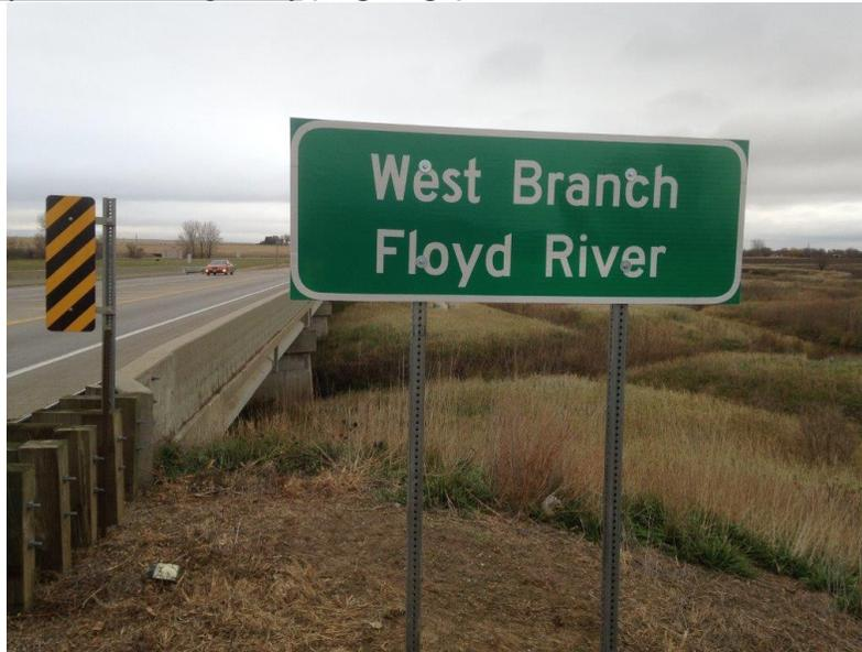
**Sign Locations:** Wherever possible, creek signs (and dual signs) should be installed in both directions of the road (a sign pair) at a creek bridge, preferably on the right side of the road in front of the bridge guardrail, as approved by the county engineer (on county roads) or by the city public works department (on city roads). Watershed signs should be installed at the river watershed divide at the entrance to the watershed (one direction of the road).
