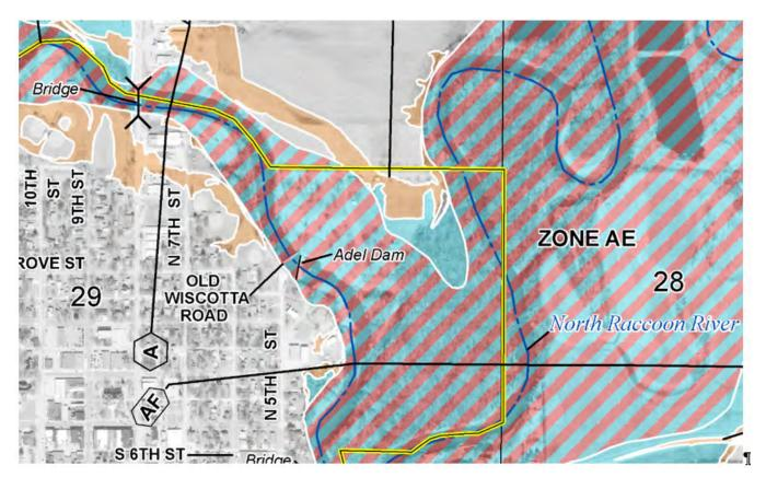
Source: Map Number 19049C0310F, Adel and Dallas Counties, Iowa – map revised Dec. 7, 2018 Figure 1-8 shows a sample from a FIRM map of Adel. Orange-shaded area = 0.2% or greater chance of flooding Blue-shaded area = 1% or greater chance of flooding Blue/red-striped area = Floodway
