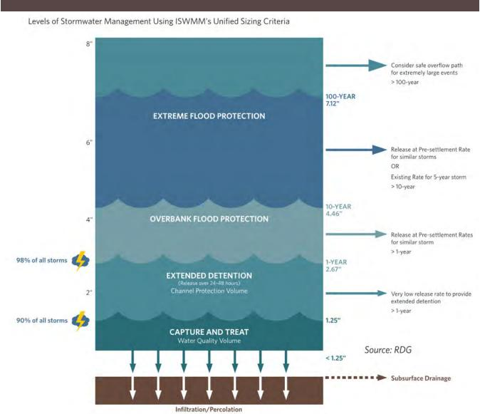
FIGURE 9-2 IOWA STORMWATER MANAGEMENT MANUAL'S UNIFIED SIZING CRITERIA (RAINFALL AMOUNTS ARE FOR CENTRAL IOWA REGION)
