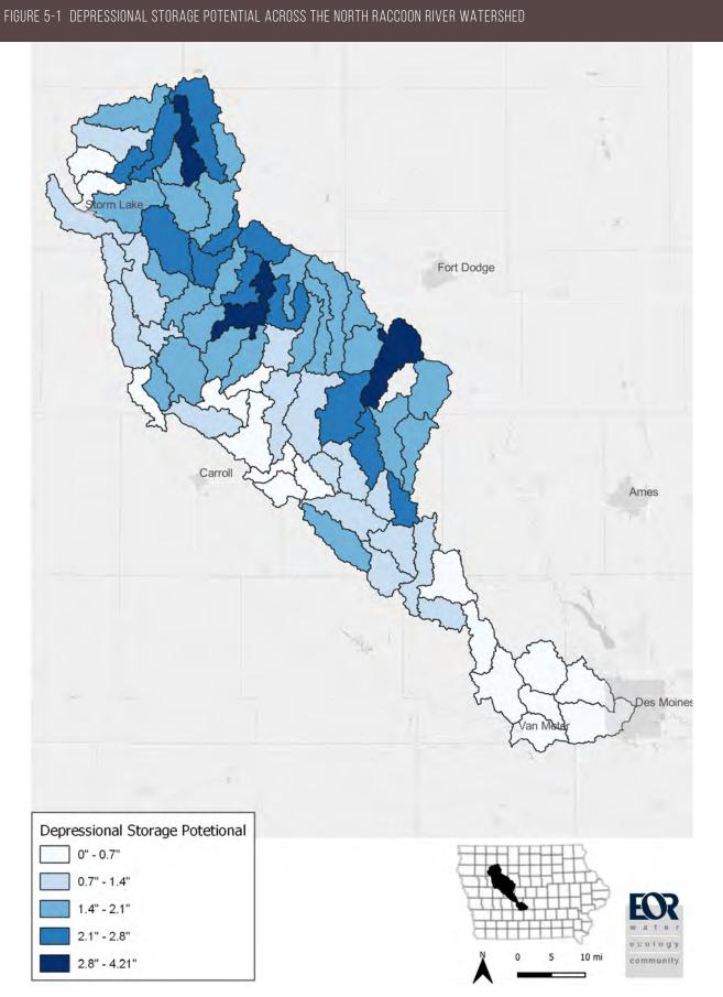
Represented in inches of subwatershed runoff. Source: EOR Analysis of Iowa Statewide LiDAR
