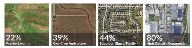
Parameters: 2.7" rainfall, 24 hour Type II rainfall distribution, Hydrologic Soil Group C soils Source: RDG 2019
