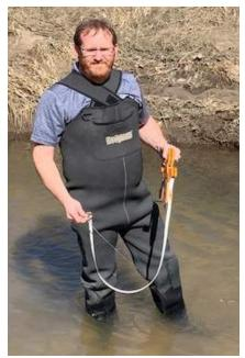
Measuring stream width during stream monitoring (City of Johnston).
