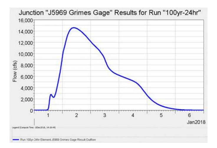
Figure 4.9: Computed HEC-HMS Peak Flow Output near Johnston, IA (called the Grimes gauge by USGS)
