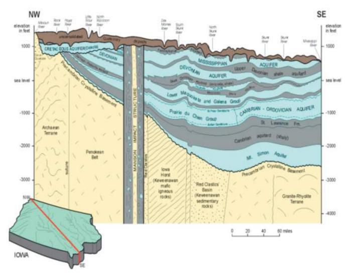
Figure 2.7: Generalized hydrogeological cross-section from northwestern to southeastern lowa (modified from Prior and others, 2003).
