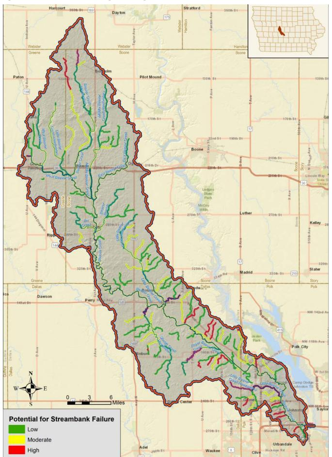
Figure 7.1: Streambank Assessment - Potential for streambank failure
