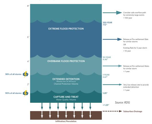
Figure 10.3 - Levels of stromwater management using the ISWMM Unified Sizing Criteria.
