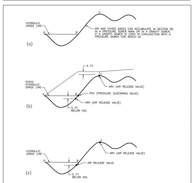
Figure 3-12 Application of air release and pressure sustaining valves (Crites & Tchobanoglous, 1998).
