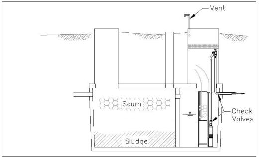
Figure 3-2 Two-compartment septic tank with turbine-style (Orenco, Inc.) pump.
