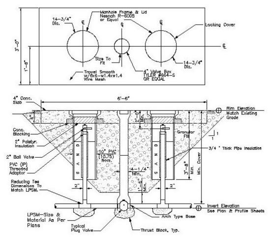
Figure 3-11 Typical dual -flush connection.
