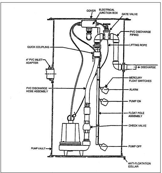
Figure 3-5 Centrifugal STEP pump in external vault. (EPA, 1991).
