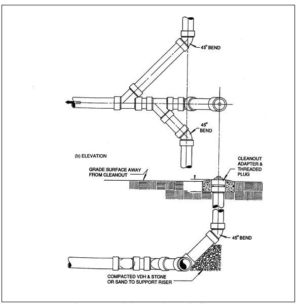
Figure 4-2 Typical STEG cleanout detail (EPA, 1991)
