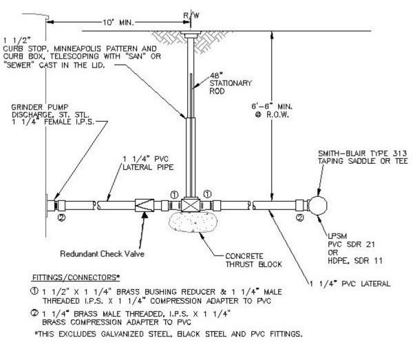
Figure 5-6 Typical curb-stop connection of a grinder station
