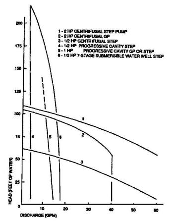
Figure 5-5 Typical discharge curves for pumps used in pressure sewer systems (EPA, 1991)
