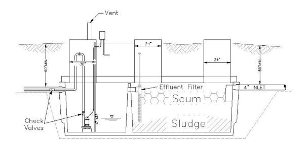
Figure 3-4 Centrifugal STEP pump and integral pump vault.
