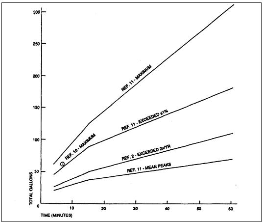
Figure 3-7 Wastewater flows for a single residence (EPA, 1991).
