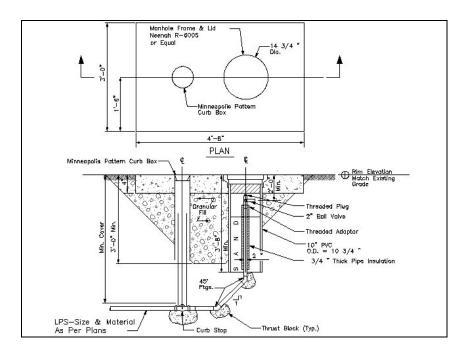
Figure 3-10 Typical single-flush connection.
