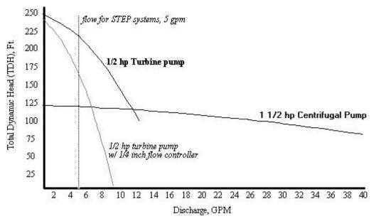
Figure 3-14 Typical pump conditions (Courtesy of Orenco, Inc.)
