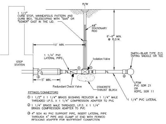
Figure 3-13 Typical STEP vault connection to forcemain.
