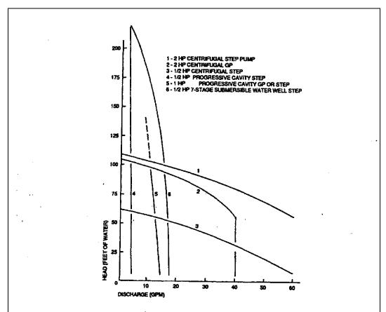
Figure 3-6 provides discharge versus head conditions for centrifugal, positive displacement, and turbine pumps (EPA, 1991).
