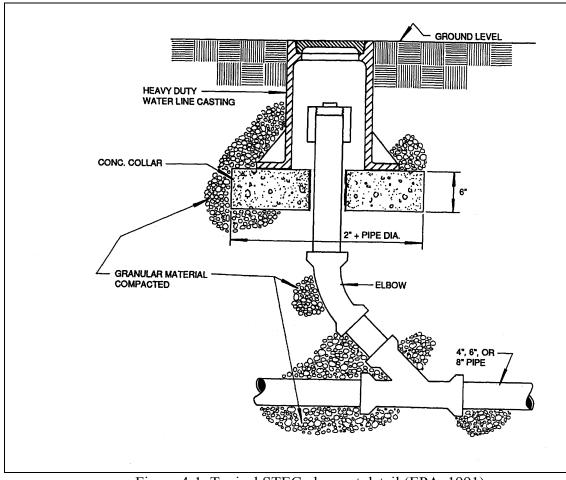
Figure 4-1 Typical STEG cleanout detail (EPA, 1991)
