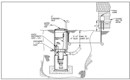
Figure 5-4 Typical Progressing Cavity Grinder Pump installation (Courtesy E/One).
