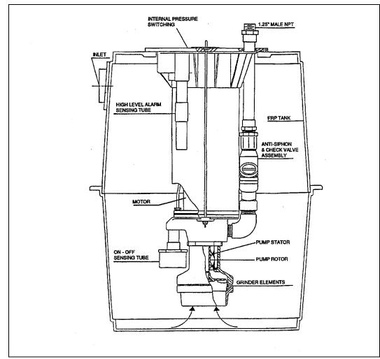
Figure 5-3 Typical Progressing Cavity Grinder Pump(Courtesy E/One).
