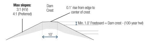
Figure 9.10-1-10: Auxiliary Spillway Parameters
