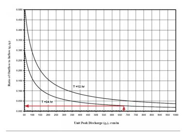
Figure C3-S6- 1: Detention time vs. discharge ratios (qo/qi)
