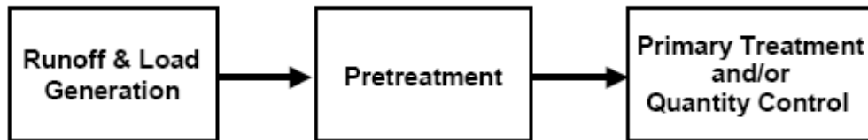
Figure C4-S3- 7: Generalized stormwater treatment train
