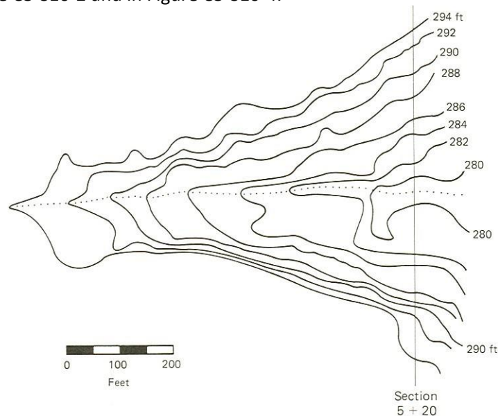
Figure C3-S10-4: Example for deriving stage-storage relationship from topographic map
