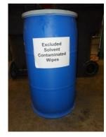
After accumulation and during transport, this same container must be sealed to meet this standard; thus, the rings must be clamped or bolted to the container.
