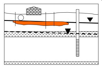
Situation III. Water Supply Well with open hole completion in bedrock but below contamination source in glacial drift.
