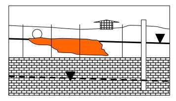
In situation I, contamination is in the same hydrostratigraphic unit as the well screen. If the well is pumped at a high rate, a risk exists that some water flowing through the contaminated zone will reach the screened interval. A Tier 3 assessment of such a
