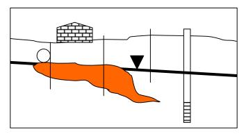
Situation II. Water Supply Well screened in confined aquifer but separated from contamination source in unconfined aquifer.
