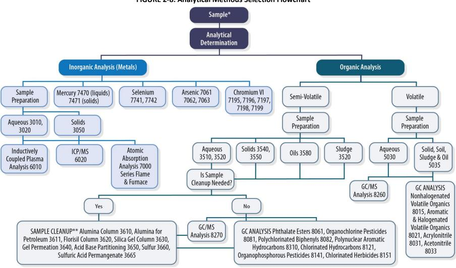
FIGURE 2-8: Analytical Methods Selection Flowchart
