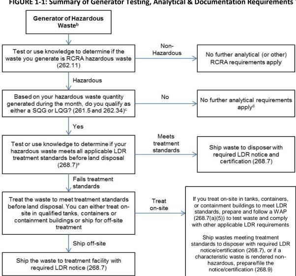
FIGURE 1-1: Summary of Generator Testing, Analytical & Documentation Requirements <sup>a</sup>
