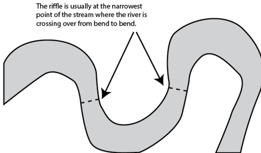
In cross-section, the bankfull width is the distance between points on opposing banks where the channel encounters its lowest floodplain. This low floodplain occurs between the one-year and two-year flood recurrence elevation. Bankfull width may be approximated using topographic data and measuring from top-of bank to top-of bank or by measuring at multiple riffles within or near the project area.
