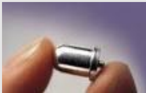
The mercury switch itself is small, about the size of a new acorn.
