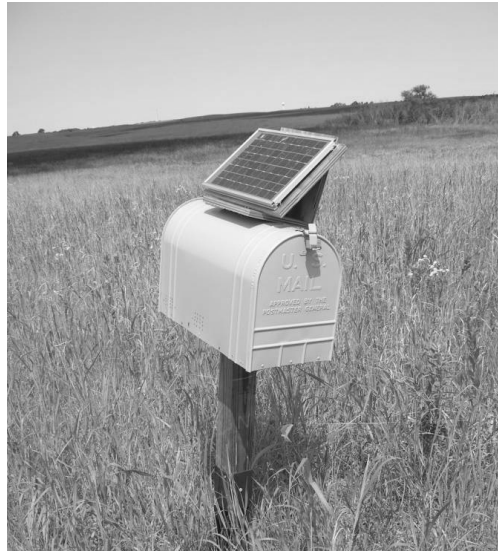
Figure 2. Henslow's sparrow playback stations established on the Spring Run Complex in 2008 and 2009. Playback stations consisted of a portable compact disc player connected to a programmable timer. Timers were connected to rechargeable 12 volt batteries and solar panels. Playback stations were mounted in aluminum boxes for protection from the elements. The aluminum boxes were drilled out in front of the player speakers to allow for sound transmission. Boxes were mounted to 4 x 4 posts at the typical perching/singing height for Henslow's sparrows in each field.
