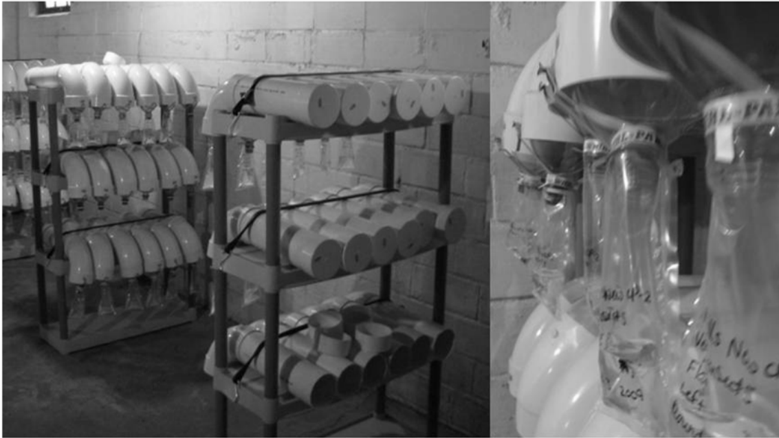
Figure 2. Invertebrate self-sorting “tubes” used to sort invertebrates collected during sweep net sampling from vegetation debris. Invertebrate samples collected during sweep net sampling were placed in 1 gallon sized zip-top bags at the completion of each survey. Sample bags were cut open and placed into the back of each tube. Invertebrate samples remained in the tubes for 24 hours. During the 24 hour sorting time, invertebrates were drawn to the light end of the tubes and were carried down a funnel into labeled whirl-pak sample bags filled with 70% ethyl alcohol for preservation. At the end of the 24 hour sorting time, vegetation and debris were removed and inspected for remaining invertebrates.
