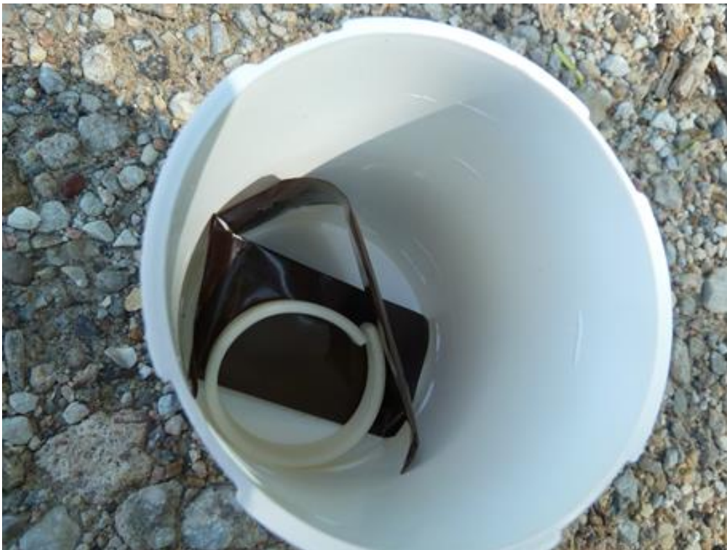
Figure 14. A look inside the Lindgren Funnel trap capture chamber. The picture shows two pheromone pouches and a 3 inch long strip of dog collar that was used to kill the beetles that entered the capture chamber. (Image: Shane Donegan, DNR)
